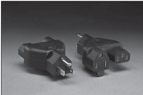
CAT. NO. 30400-B NEMA 5-15P, IEC 60320 C-13 (X1), NEMA 5-15R (X1) PLUG, CONNECTOR ADAPTER, 10 A-125 V.
